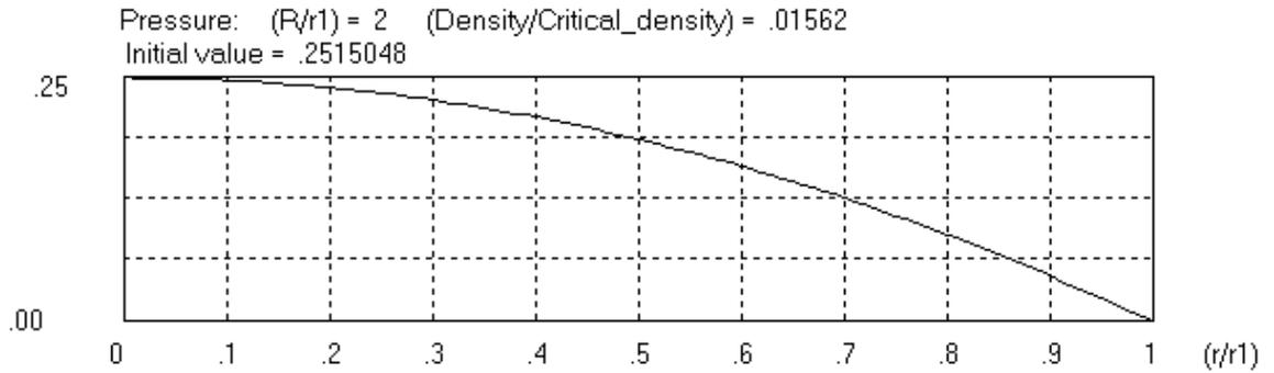
Figure 2. The distribution of the pressure far from the collapse
