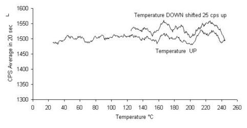
Figure 6 - Test of chip 2, LiF200, 2 Gray, PMT 2, with heat, 2006 Signal on Slave Chip (not heated). Master chip heated 4 m away.
