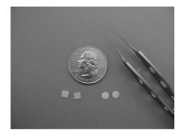
Figure 3: Chips LiF 100 are shown to the left, chips LiF 200 to the right, the coin is a quarter dollar.
